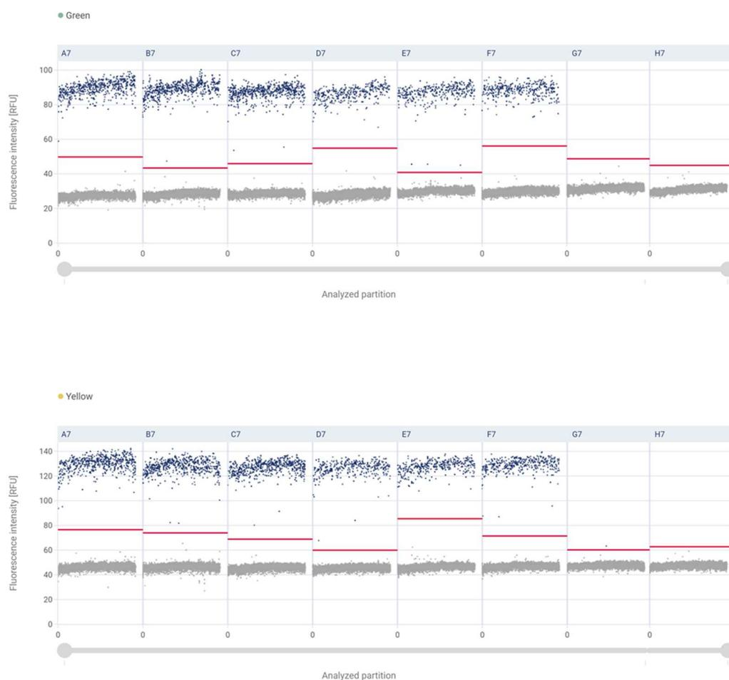
**2D Scatter Plot:** Single-well data of target assay TRIO (Green Channel, X-axis) and reference assay TERT (Yellow Channel, Y-axis) in 4ng gDNA input amount.
