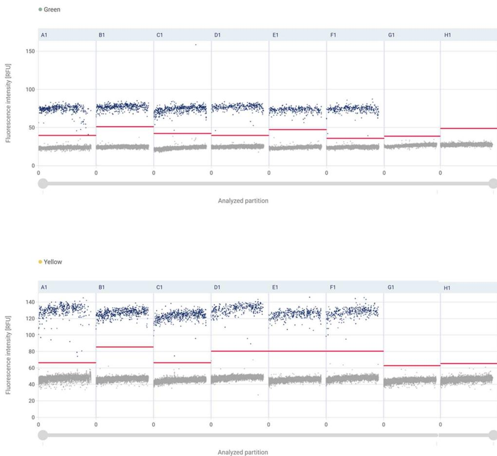
**2D Scatter Plot:** Single-well data of target assay LIPA (Green Channel, X-axis) and reference assay TERT (Yellow Channel, Y-axis) in 4ng gDNA input amount.
