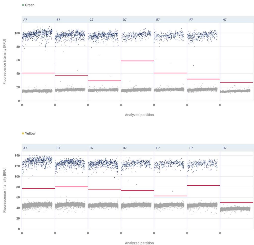
**2D Scatter Plot:** Single-well data of target assay DUSP6 (Green Channel, X-axis) and reference assay TERT (Yellow Channel, Y-axis) in 4ng gDNA input amount.
