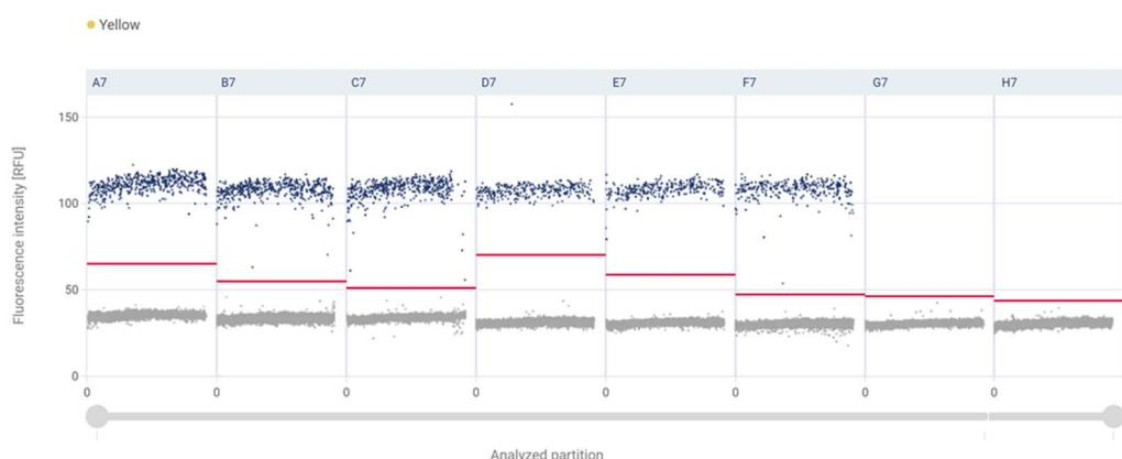
**2D Scatter Plot:** Single-well data of target assay FANCA (Green Channel, X-axis) and reference assay AP3B1 (Yellow Channel, Y-axis) in 4ng gDNA input amount.
