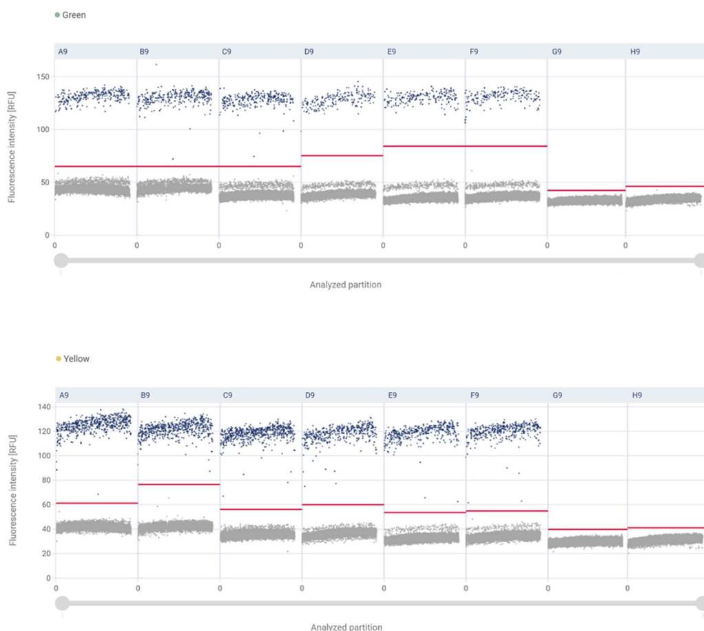
**2D Scatter Plot:** Single-well data of target assay PLP1 (Green Channel, X-axis) and reference assay TERT (Yellow Channel, Y-axis) in 4ng gDNA input amount.
