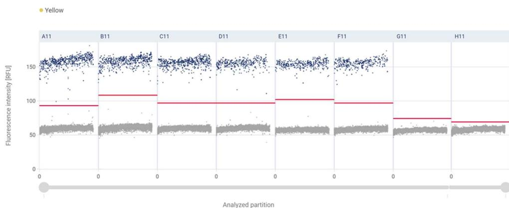
**2D Scatter Plot:** Single-well data of target assay NOTCH2 (Green Channel, X-axis) and reference assay TERT (Yellow Channel, Y-axis) in 4ng gDNA input amount.
