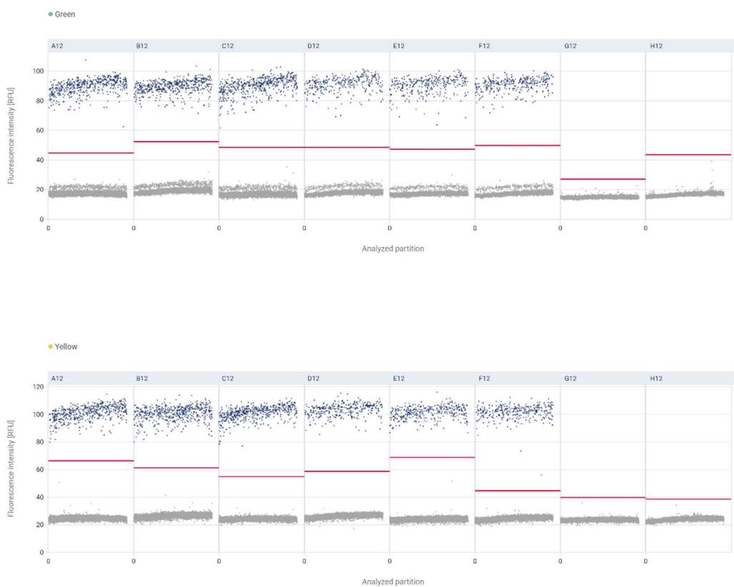
**2D Scatter Plot:** Single-well data of target assay ALK (Green Channel, X-axis) and reference assay AP3B1 (Yellow Channel, Y-axis) in 4ng gDNA input amount.
